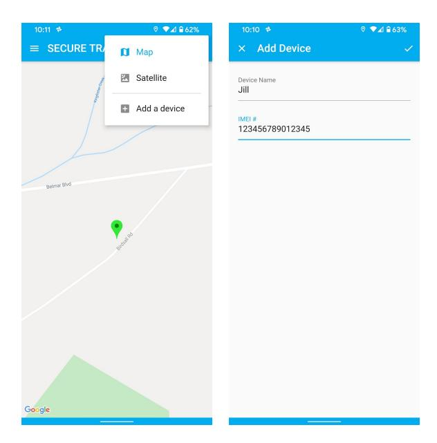
**NOTE:** After you add your device you may need to restart it before it shows online by sending the command **RESET#** to the device's phone number by text message, or using the pinhole inside the phone above the SIM card to the right of the round button.
